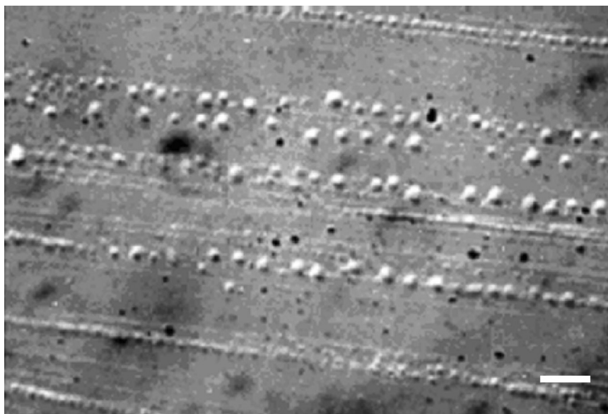
FIGURE 8 Optical microscope image of Rh6G self-assembled array specimen embedded in a transparent polymer PMMA film.
